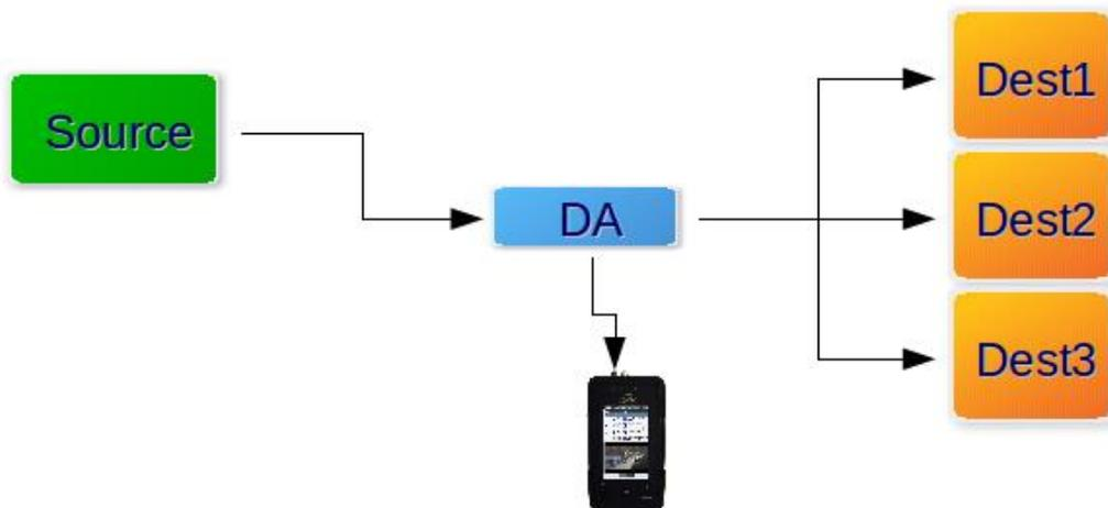
If no distribution amplifiers are used, most analyzers allow the signal to be looped through the device so that it can be inserted in-line between points of interest to determine the problem area.
